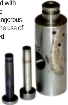
Parts damaged and overheated (discolored) from diesel fuel with poor lubrication.
