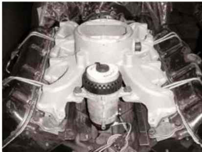
Illustration shows 6.5L filter assembly for P-Chassis Vehicles. The 6.2L filter assembly is a different square-like shape.
